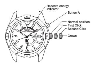
SEIKO KINETIC watches are marvels of brilliantly applied technology. They convert energy created by the movement of the wrist into electricity which is stored, regulated and released with perfect quartz accuracy. No need to ever change a battery.
