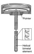
Fig. 6.6.8 - A kitchen thermometer is based on a bimetallic strip that has been wound into a helix. As the temperature changes, the helical element coils or uncoils and turns the pointer.
