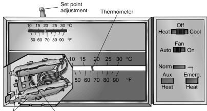
Mercury tilt switches Bimetallic coil temperature sensor
