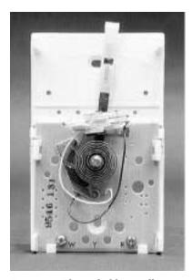
Fig. 6.6.9 - The coiled bimetallic strip in this home thermostat controls the orientation of a mercury tilt switch. As the ball of liquid mercury tips from one end of the glass switch to the other, it turns the furnace on or off.
