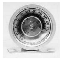
Fig. 6.6.7 - This refrigerator thermometer uses a coiled bimetallic strip to measure temperature. The coil unwinds as it cools.
