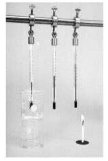
Fig. 6.6.2 - As their temperatures increase—from left to right—both the glass and the liquid in these thermometers expands. However the liquid expands more and flows up the tube inside the thermometer.
