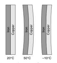
Fig. 6.6.6 - A copper and an iron strip are bonded together to form a bimetallic strip. Since copper has a larger coefficient of volume expansion than iron, the strip curls in response to changes in temperature. The strip's shape is an accurate indication of its temperature.
