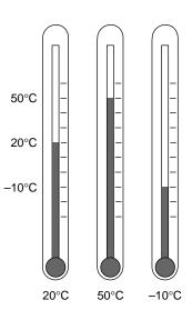
Fig. 6.6.3 - The liquid inside a glass thermometer has a larger coefficient of volume expansion than the glass. As the temperature increases, excess liquid is driven out of the cavity at the base of the thermometer and the thin column of liquid in the capillary rises. As the temperature decreases, liquid returns to the cavity and the column falls.
