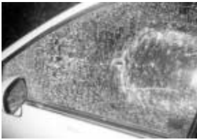
Fig. 16.2.9 - When a small rock cut through the compressed outer skin of this tempered glass car window, it exposed the tense inner layer. That layer immediately began to tear and the entire window broke into thousands of tiny fragments.
