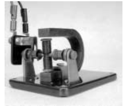
Fig. 9.5.2 - Current flows into and out of the rotor of this DC motor through the metal brushes on the left. These brushes touch the rotor's commutator so that current in the rotor's coil reverses every half turn.
