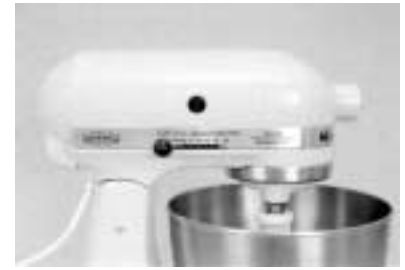
Fig. 9.5.5 - The top of this kitchen mixer contains a universal motor, which turns the mixing blade through a series of gears. The motor's graphite brushes can be serviced through black plastic ports, one of which is visible near the center of mixer. The speed switch controls the current to the motor.
