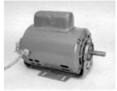
Fig. 9.5.8 - This 1 horsepower (750 W) induction motor is used in industrial and commercial equipment. The projection on top contains a capacitor that helps produce the rotating magnetic field the motor needs to spin its rotor.
